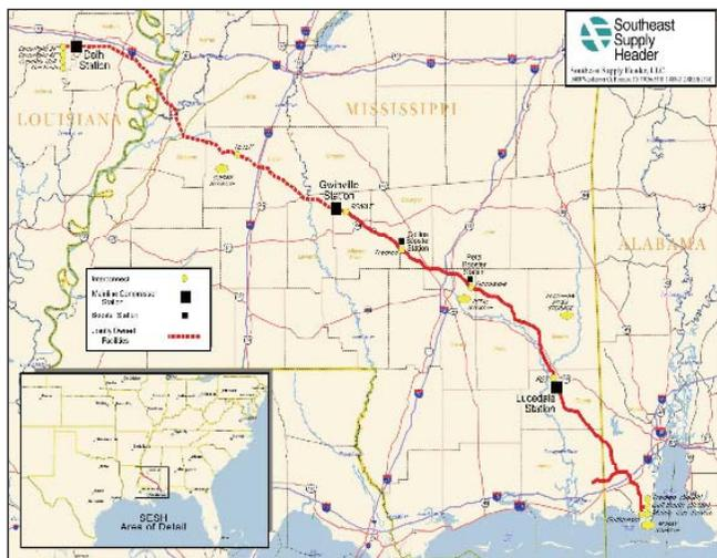
Other significant projects include the Southeast Supply Header (SESH) that is being built for Southeast Supply Header LLC, a joint venture of Sempra Energy and CenterPoint Energy. Consisting of 270-miles of 42- and 36-inch pipe, the SESH will begin near the Perryville Hub in northeast Louisiana and connect with the Gulfstream Natural Gas System LLC pipeline in Mobile County, AL. The new line's capacity is projected to reach 1 Bcf/d and begin service by mid-summer 2008.
